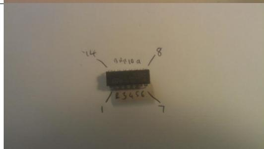
Put it in the breadboard so it straddles the central groove. Push it in so that pin 1 is in location E9 and pin 8 is in F15.
