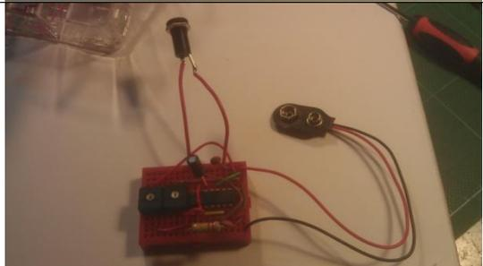
Congratulations! You have now finished your first noise box! Now, the moment of truth... does it work? Attach the audio cable which is connected to the test speaker to the output jack, then connect the 9 volt battery, and....
