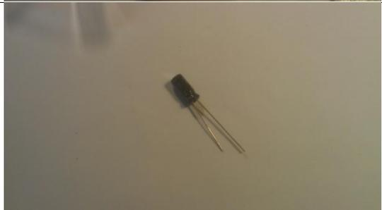
Connect the long leg - the positive one - to the positive rail at G16. Then connect the short leg to the mini-jack socket by plugging it into I8.
