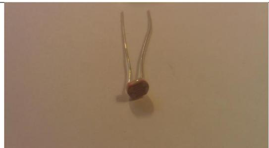
Try plugging it in between the power rail and one of the pots, then you can control the pitch or pulse width by waving a light at it or covering up the LDR. Congratulations - you've started hacking!
