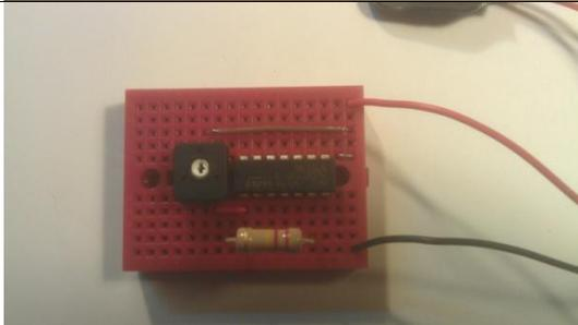
Now we need to connect pins 2 and 6. Do this with a yellow jumper wire from D11 to D14.
