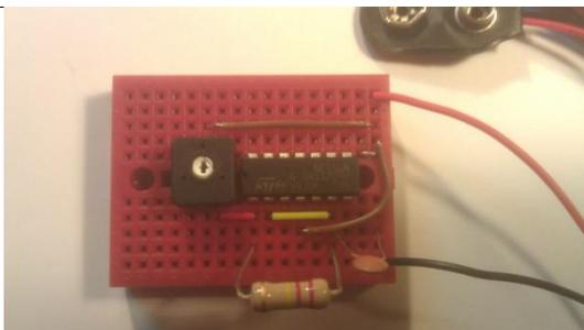
Pin 5 needs to be connected to Pin 8, so plug a jumper wire into B13 and join it to G15.
