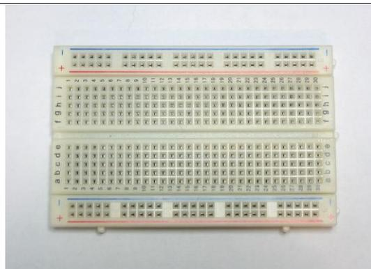
Most regular sized breadboards look like the one on the right. The top 2 and bottom 2 horizontal rows of holes are all connected underneath the breadboard, and each of the 5 vertical columns of holes are connected. So, thinking of things a bit like a game of Battleships, if you plug one component into 'A1' and one into 'E1' then they will be connected as if they were soldered together.
