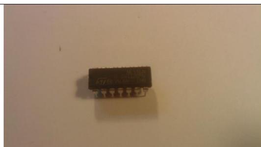
This means pin 1 is in the bottom left corner, and then counting anti-clockwise, pin 7 is bottom right, pin 8 is top right and pin 14 is top left.
