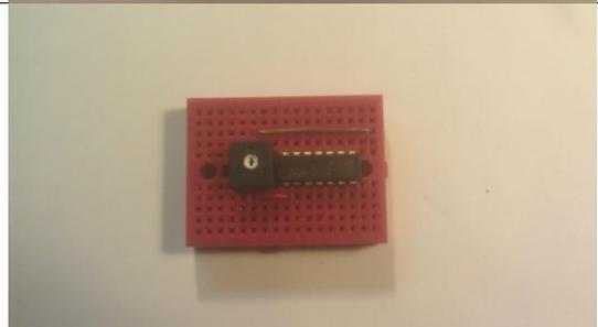
Now we are going to turn the top columns (F-J) 16 & 17 into the 'positive rail' and the bottom column 17 (A-E) into the 'ground rail'.
