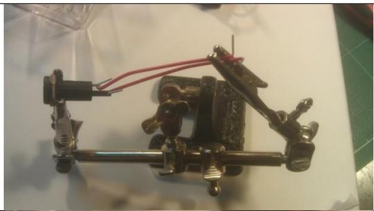
Then you need to solder the wires onto the socket. Heat the **wire** and then push the solder against the heated wire until it melts. Then remove the solder but leave the soldering iron on for a couple of seconds, then remove the soldering iron. If this is your first go at soldering, don't be afraid to ask for help. There is some extra info on soldering at the end of this guide.
