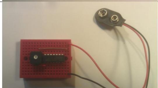
Because we need more than 4 holes for positive connections, we're going to 'bridge' two columns with a small jumper. Push the tiniest jumper wire in to connect F16 and F17.
