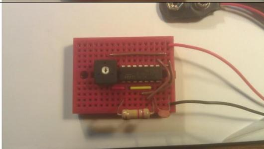
Now it starts to get fiddly...Pin 7 needs to go direct to the ground rail. Plug a jumper wire from C15 - D17... or anywhere in the lower half that connects 15 to 17. In fact by now you might have worked out that it doesn't need to be that *exact* hole, just somewhere in that column of 5 holes.
