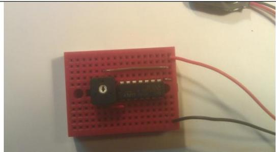
Next to connect pins 1 and 6 with a resistor – it's the beige thing with paper on the end. Remove the paper and fold the wires at 90 degrees.
