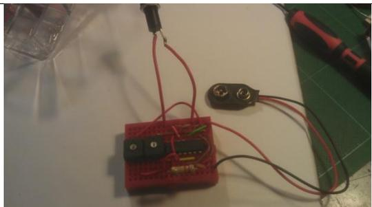
Then we need to connect the socket to the positive rail via a capacitor. This time we're using the black barrel-shaped one, and it *does* matter which way round it goes.
